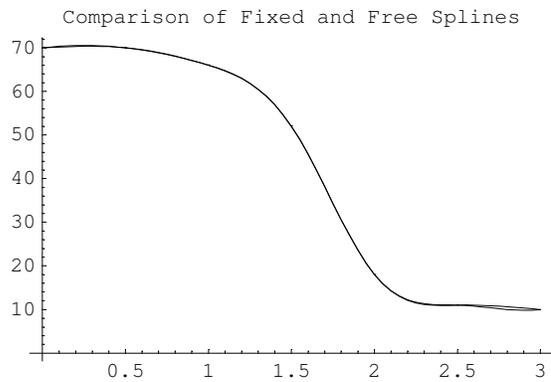
For this example, the only difference occurs near the end points. For the above, `FreeSplinePlot` and `FixedSplinePlot` were created using the procedure `PiecewiseCubicPlot` and a scrap sheet.
